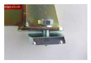
You can probably see how the brackets fit- they sit on top of the raised lips on your van with the threaded nut plate underneath the lip and an M8 bolt and spring washer through the top of the bracket. There's no need to over-tighten anything- once the spring washers are flat and the bracket is secure, you're good to go.
